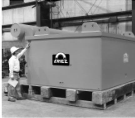
Hundreds of manually cleaned Eriez units are in service throughout the world. They are ideal for installation where protection is needed to catch the occasional piece of iron that might contaminate the material flow. This specially designed magnet weighing 65 tons is used over a copper ore conveyor located in Chile.
